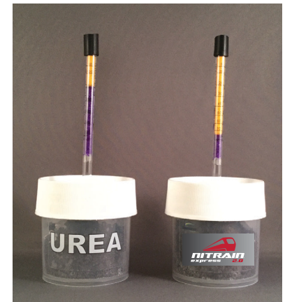
48-Hours After Application Significantly less N loss with Nitrain Express 2.0 as demonstrated by lower amount of ammonia detected by Dräger tube
